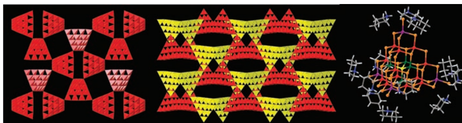
Figure 1. The structures of OCF-1, OCF-5, and OCF-40. The disordered amine template molecules in OCF-1 and OCF-5 are omitted for clarity. Red spheres stand for Ga, yellow for S, green for Zn, purple for Sn/Ga, orange for Se/S.
